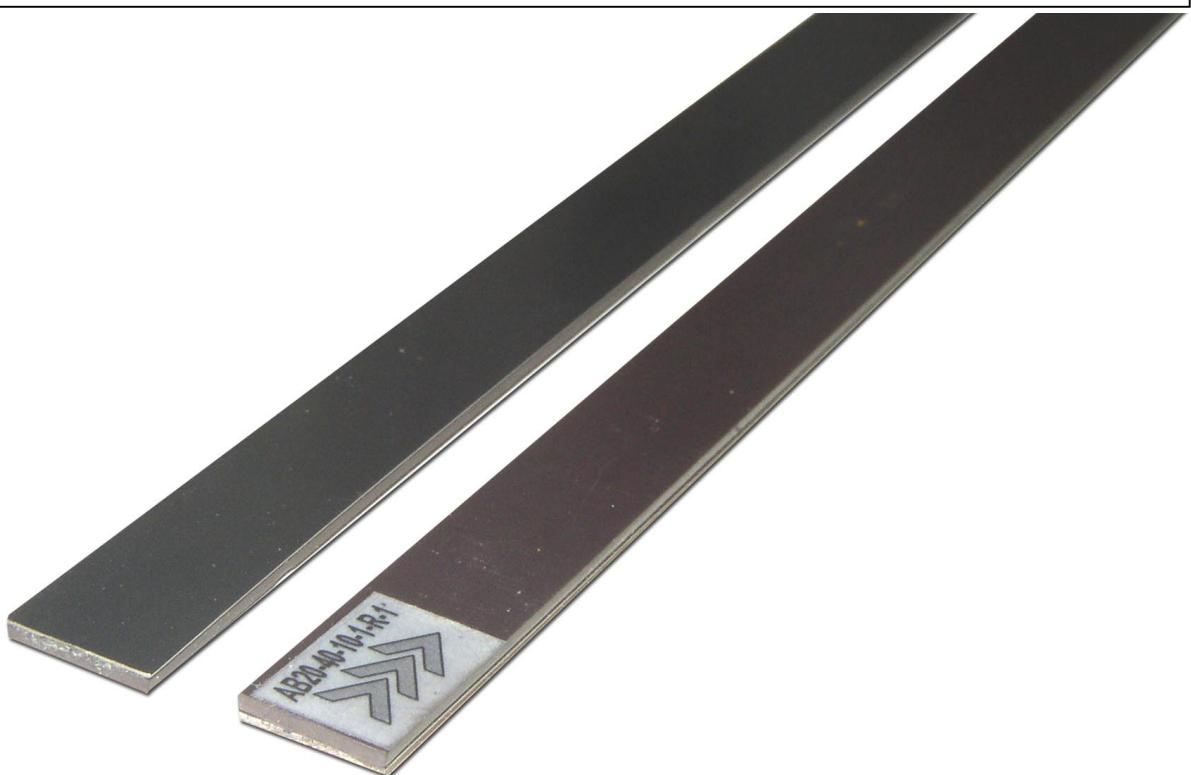
The ELGO magnetic tapes contain digital information, which are necessary for magnetic measurement by ELGO linear encoder types, either as an incremental or absolute code. The tape must be installed along the measuring distance and can be stuck (standard tape construction R) or can also be installed owing to its own magnetization on ferro-magnetic surfaces (when ordered tape construction A).
